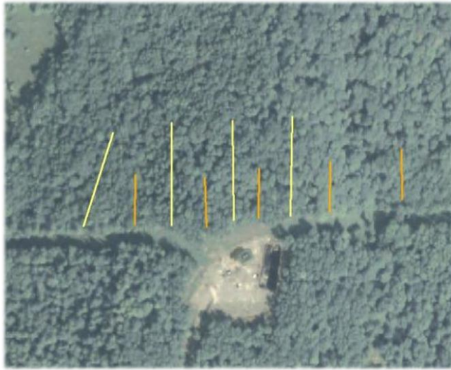
Figure 2. Natural cover transects (yellow) begin at the pipeline edge and extend 100 m into the forest. Artificial cover transects (orange) begin at the edge and extend 50 m
