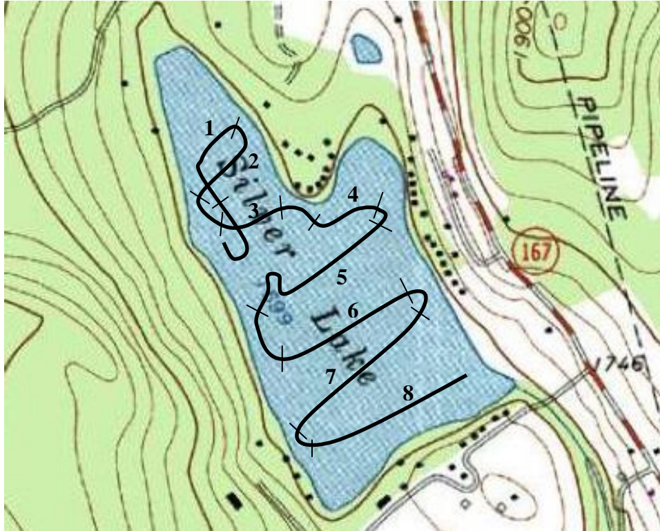
Figure 6. Approximate track taken during hydroacoustic survey and locations of transects 1 through 8 surveyed in Silver Lake on October 14, 2008.
